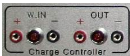
[Input and output terminals of Charge controller]
