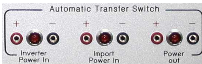
[Inverter & Import power input terminals and output terminals]
